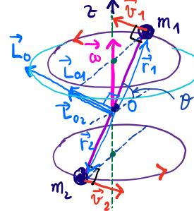
Si calcola  $\vec{L}_o = \vec{L}_{o1} + \vec{L}_{o2}$ ,  $\vec{L}_{oi} = \vec{r}_i \times \vec{p}_i = m_i \vec{r}_i \times \vec{v}_i = m_i \vec{r}_i \times (\vec{\omega} \times \vec{r}_i) = m_i \omega \cos \theta r^2 \hat{u}$
