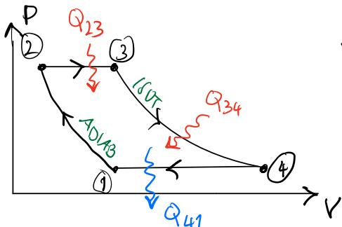
$$W_{\text{TOT}} = Q_{\text{TOT}} = \underbrace{Q_{23} + Q_{34}}_{\text{assorb.}} + \underbrace{Q_{41}}_{\text{ceduto}}$$
