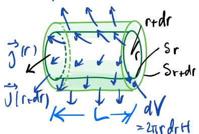
$$S_r \dot{q}_r - S_{r+dr} \dot{q}_{r+dr} \approx -2\pi L \left[ \dot{q}_r + r \frac{\partial \dot{q}_r}{\partial r} \right] dr = d\dot{Q} = dM \cdot c_v \frac{\partial T}{\partial t} = p \cdot c_v dV \frac{\partial T}{\partial t} = 2\pi r L p c_v \frac{\partial T}{\partial t} dr$$
