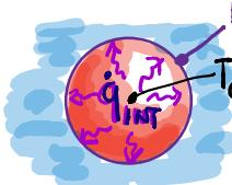
Si utilizza ancora la  $\rho c_p \frac{\partial T}{\partial t} = \frac{1}{r^2} \frac{\partial}{\partial r} \left( k r^2 \frac{\partial T}{\partial r} \right) + \dot{q}_{\text{int}} = 0$
