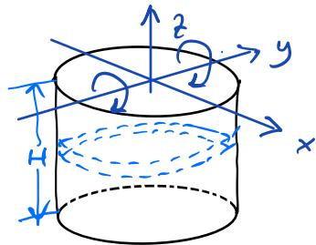
$$dI_{\text{ANELLI},y} = z^2 dm + \frac{R^2}{2} dm \quad \text{dove } dm = \rho_{\text{LAT}} \cdot 2\pi R dz \Rightarrow$$
