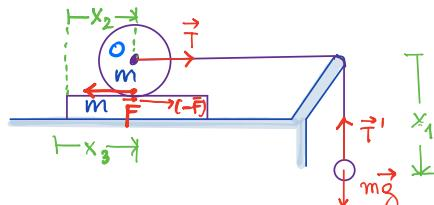
$$I_0\ddot{\theta} = FR \text{ con } R\ddot{\theta} = \ddot{x}_2 - \ddot{x}_3, I_0 = \frac{mR^2}{2}.$$
