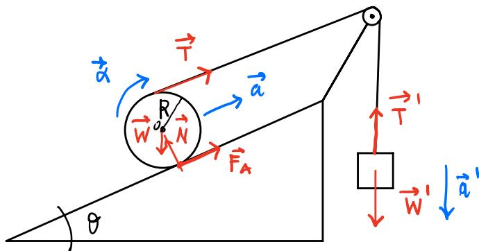
$$|\vec{T}| = |\vec{T}'| ; \quad W = Mg, \quad W' = mg$$
