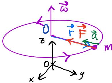
$$\begin{aligned} \vec{F}' &= \vec{0} \\ \vec{a}' &= \vec{0} \\ \vec{F}_A &= \vec{F} = \\ &= -m\vec{\omega} \times (\vec{\omega} \times \vec{r}) \end{aligned}$$
