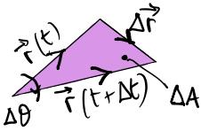
$$\Delta A = \frac{1}{2} |\vec{r}(t+\Delta t) \times \vec{r}(t)| ; \quad \vec{r}(t+\Delta t) - \vec{r}(t) = \vec{v}_n(t) \cdot \Delta t \Rightarrow \vec{r}(t+\Delta t) = \vec{r}(t) + \vec{v}_n \Delta t$$
