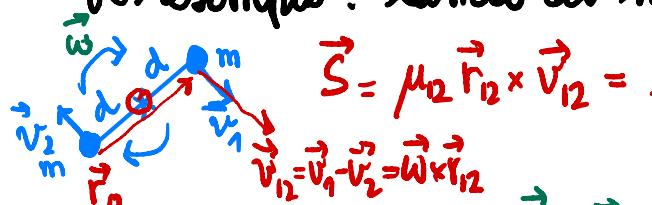
$$\vec{S} = \mu_{12} \vec{r}_{12} \times \vec{v}_{12} = \frac{m}{2} (2d)(2d) \vec{\omega} = (2md^2) \vec{\omega}$$
