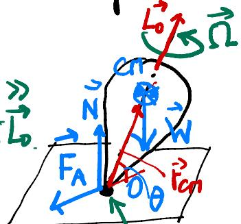
$$\Delta L_0 \approx L_0 \cos\theta \cdot \Delta\phi = T_0 \Delta t = r_{cm} Mg \cos\theta \Delta t$$
